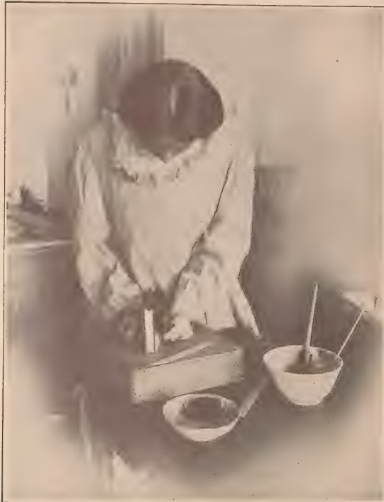
No. 13—Stretching leather over back of book on paring stone
